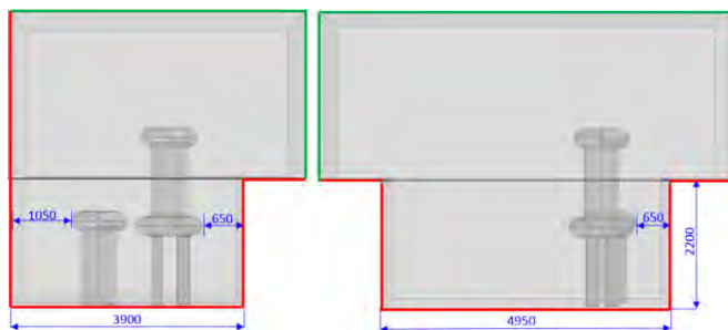
Fig. 4. Selected dimensions of the fenced test field at HV Lab at AGH-UST and location of the cascade transformers (left - front view, right - side view)
